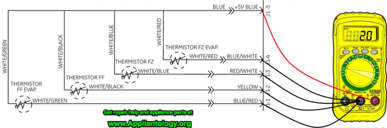
Typical voltage drop is between 1 to 4 dc volts. A thermistor voltage drop of 0vdc indicates a shorted thermistor, 5vdc would indicate an open thermistor. Any voltages below 1vdc or above 4vdc could indicate a suspect thermistor, follow up with a direct test of the thermistor.
